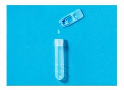
Open the pack with the buffer and pour it into the tube.
